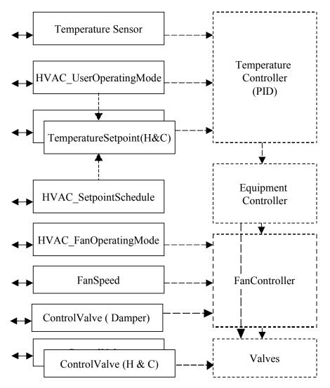
Solid lines indicate interfaces exposed via UPnP Dotted lines indicate interfaces and services not directly visible via UPnP
